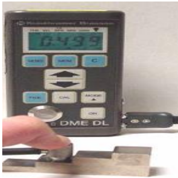
Figure 01. Calibration of ultrasonic thickness gauge using the test block
